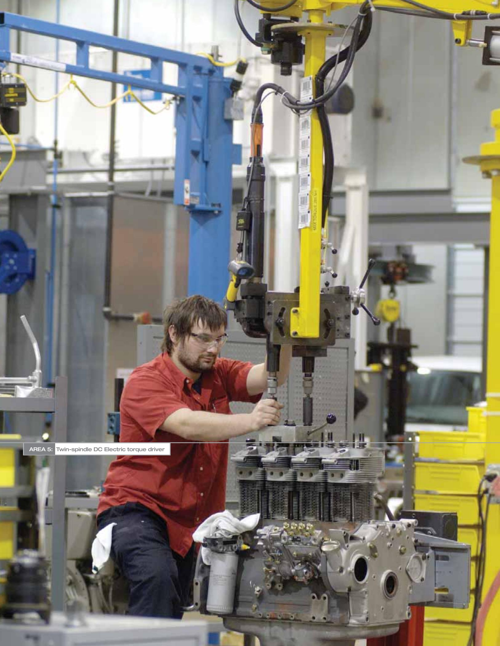
AREA 5: Twin-spindle DC Electric torque driver
